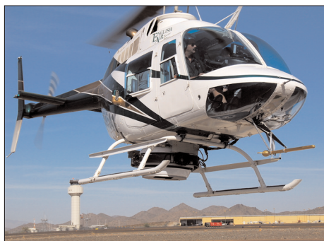
Corridor mapper mounted under helicopter. (See page 451/ voir page 451.)
